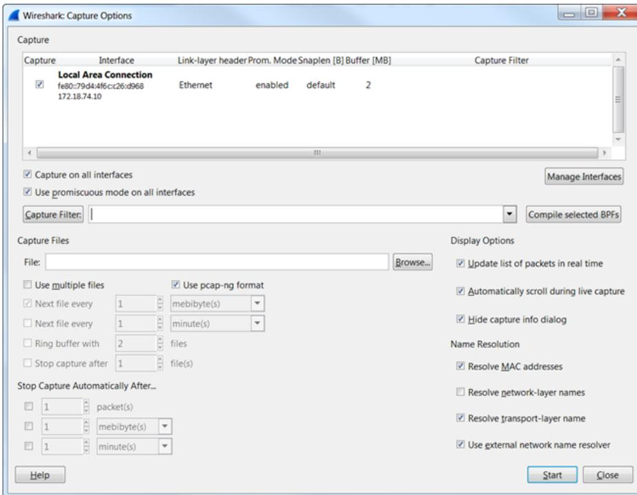
This Capture Options dialog should display your Ethernet interface. Make sure that the “Capture on all interfaces” and “Use Promiscuous Mode” boxes and the “Update List of Packets in Real Time” and “Automatically Scroll during Live Capture” boxes are checked.
