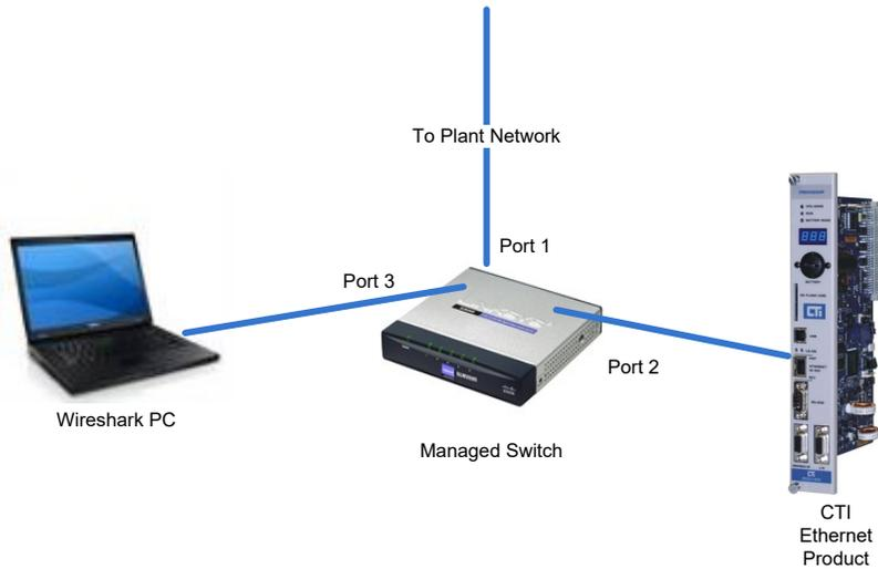
Figure 1. Network Capture Setup
