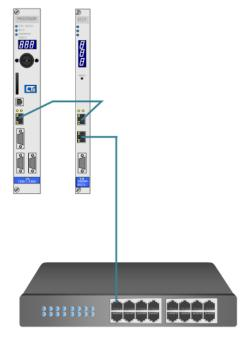
All communication devices will be connected to the Ethernet switch or to other switches in the network
