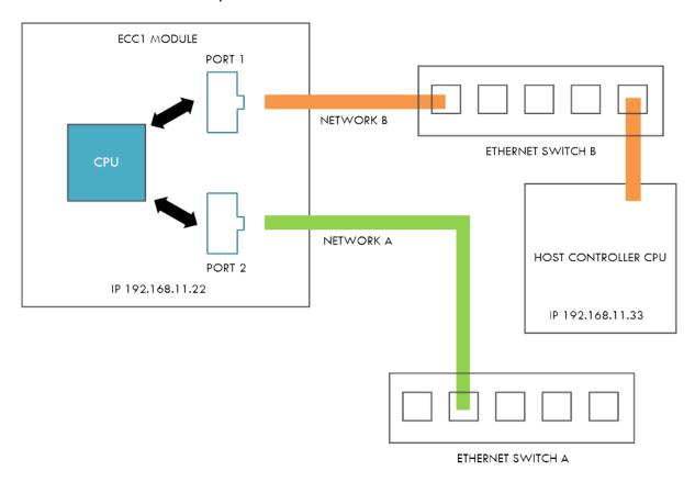
In this configuration the 2 networks connected to port 1 and port 2 are independent.
