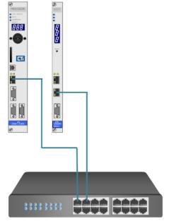
Using this method, all communications between the HMI and the 2500P-ECC1 module and between the 2500P-ECC1 module and the 2500 Series® controller pass through the network switch. In addition, communications between the programming workstation and the 2500 Series® controller pass through the network switch.
