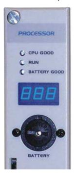
The IP address is displayed on the Multi Segment Display on the Front Panel. The 4 octets of the IP address are cyclically displayed one after the other, separated by a dot after the lowest octet.
