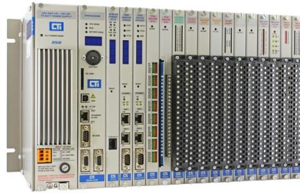
Figure 2: CTI 2500 Series® 16-slot rack
