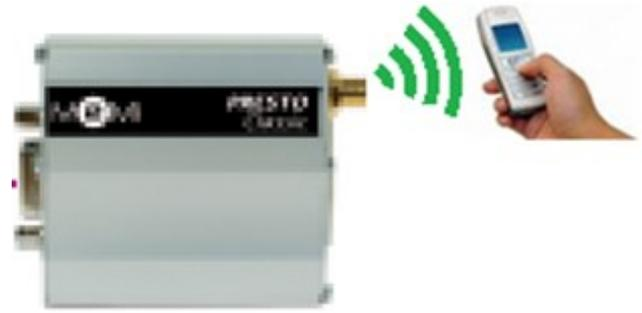
*The Message Control feature in zenon allows sending an SMS (or email) via a modem with a SIM card to alert maintenance crew agents when an alarm or an abnormal event occurs.*
