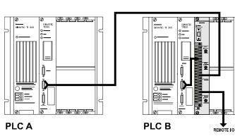
The remote I/O port of PLC A and PLC B are both connected to the appropriate terminals on the RPM. The cable from the remote I/O is connected to the module. Three sets of nine additional terminals are provided for switching the connections between operator interface devices and the PLC communication ports. These connections are not shown in the figure above. See wiring diagram on back page for details.
