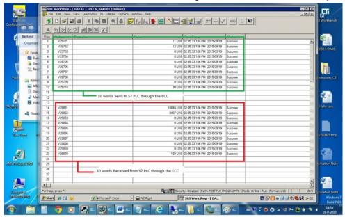
Data window in the S7 PLC with the Configured communication memory area.
