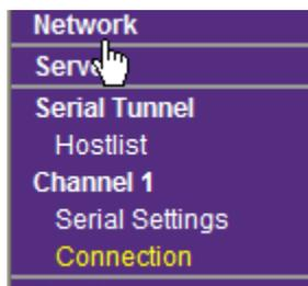
Here you will enter the information for the connection to the 2572-A. Under Endpoint Configuration is where you setup the Remote Port and Remote Host. The Remote Port is the port number of the 2572-A, this is always 1505. The Remote Host is the IP address of the 2572-A. When finished click OK.
