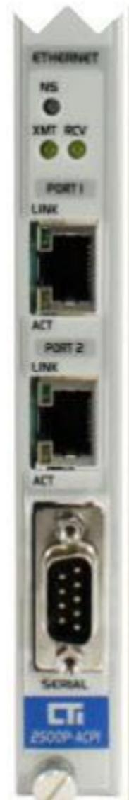
Each Ethernet port connector contains two embedded LEDs. The **LINK** LED indicates whether the Ethernet port is successfully connected to another Ethernet device, such as a network switch. The **ACTIVITY (ACT)** LED provides visual indication that Ethernet packets are being received or transmitted via the port. See the following table below for more information.
