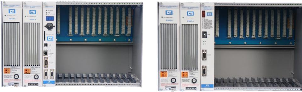
**Power supply redundancy for CPU and RBC**
