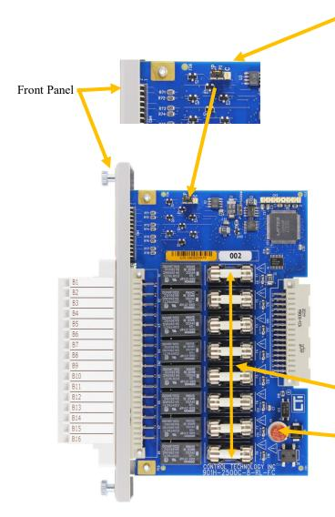
Module Logon Selection Jumpers. CP or Classic Plus mode. CP or Classic Plus mode is the default shipping configuration. In CP mode the module logs in as a 8X/8Y for blown fuse reporting. In C or Classic Mode the module logs in as a 8Y and does not provide blown fuse reporting. This allows customers to modify the module logon based on their application requirements. JP2 is available only on 901C Rev boards or higher.
