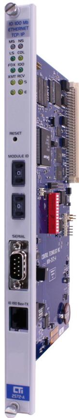
The CTI 2572-A module directly attaches to Ethernet twisted pair cabling via the Ethernet CAT5e connector (RJ-45) and can be used with either 10Mb or 100Mb data links (half or full duplex operation). The module automatically detects network speed and duplex mode and configures its port accordingly. The firmware includes a full function TCP/IP stack that supports both TCP and UDP protocols.
